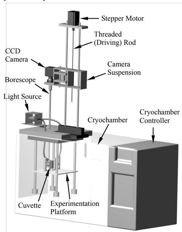
Figure 1: Graphical illustration of the cryomicroscope, integrated with a controlled-rate freezer [4].
