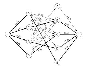
Figure 3.4. Graph  $G_{\text{minweight}}$  for the minweight\_alldifferent constraint of Example 3.12. For each arc a, (c(a), w(a)) is given. Bold arcs indicate a minimum-weight s - t flow with weight 21.
