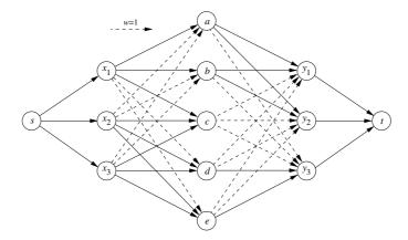
Figure 4.12. Graph representation for the variable-based soft\_same constraint. For all arcs the capacity is 1. Dashed arcs indicate the inserted weighted arcs with weight 1.
