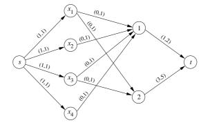
**Figure 4.4.** Graph representation for the gcc. Demand and capacity are indicated between parentheses for each arc a as (d(a), c(a)).
