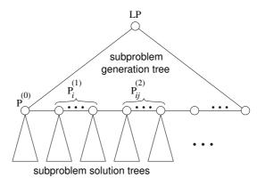
**Figure 6.1.** The structure of the search tree. The linear programming relaxation LP is located at the root. The subproblems  $P^{(k)}$  correspond to discrepancy k.
