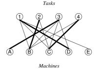
Figure 3.1. The value graph for the task assignment problem of Example 3.1. Bold edges form a matching covering all tasks.
