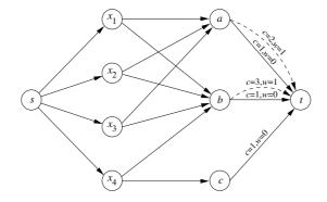
Figure 4.2. Graph representation for the variable-based soft\_alldifferent constraint. For all arcs the capacity c = 1, unless specified otherwise. Dashed arcs indicate the inserted weighted arcs with weight w = 1.
