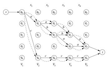
Figure 4.9. Graph representation for the variable-based soft\_regular constraint. For all arcs the capacity is 1. Dashed arcs indicate the inserted weighted arcs with weight 1.
