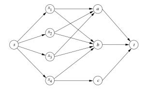
Figure 4.1. Graph representation for the alldifferent constraint. For all arcs the capacity is 1.
