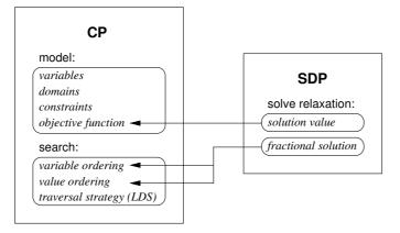
Figure 7.1. Communication between constraint programming (CP) and semidefinite programming (SDP).
