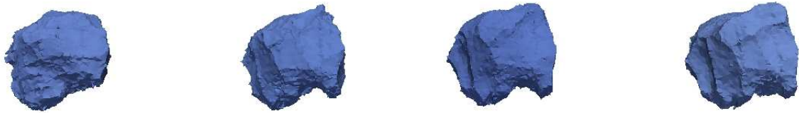
Figure 5.18: Single grain extracted from the meshes in Figure 5.8. The anneal state increases from left to right, with the initial state on the left. The grain increased by 25% in volume from the initial to third anneal state and is one of the larger tracked grain with \bar{R} = 109\mu\text{m} (see Section 5.7.2).
