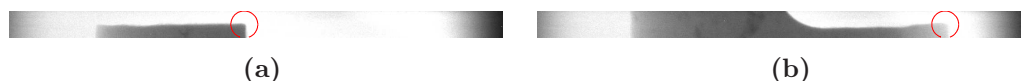
Figure 5.1: Profiles of the tip of the nickel sample in the transmitted beam. Images are the result of translating the sample vertically by 1 mm, with (a) as the top projection and (b) the transition region into a full cylinder. The red circles indicate the reference position that was used for determining geometrical changes in the sample as well as marking the vertical displacement required to collect overlapping sample volumes. In the fourth anneal state, the sample began to exhibit a bow, which resulted in the distance between the two recorded circles to expand. Hypotheses concerning the origin of this bowing are discussed in the text.
