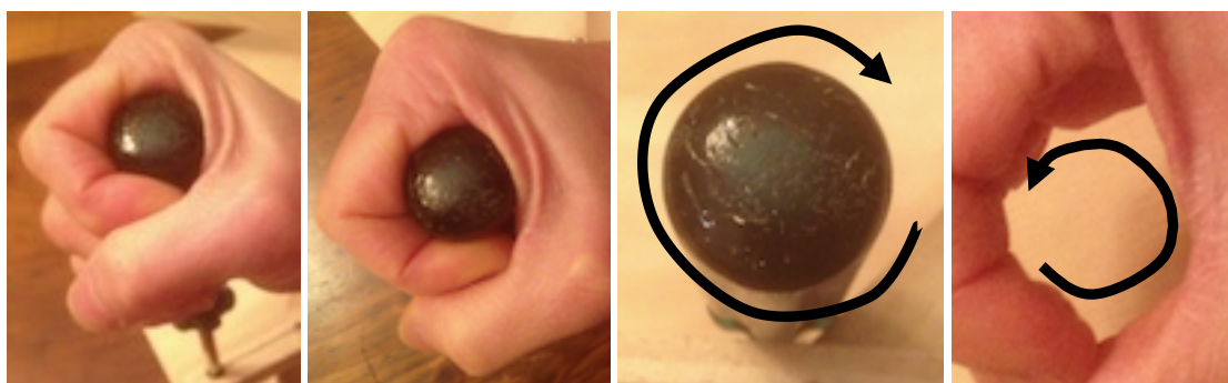
Figure 3. Photos and representation of a couple between hand and screwdriver
