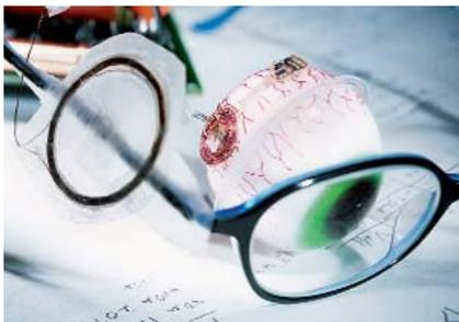
be packaged and worn on a belt—would send images wirelessly from the camera to the implant in his or her eye. "Here's the transmitter coil," Wyatt says, pointing out two concentric copper rings taped to the earpiece of the glasses. Using radio waves, he says, the inner ring sends the data to the prosthesis, while the outer coil sends it power.
