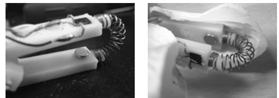
Fig. 1. (a) Real image of the anal sensor. (b), (c) Detail images of a hall-electrode and magnet.
