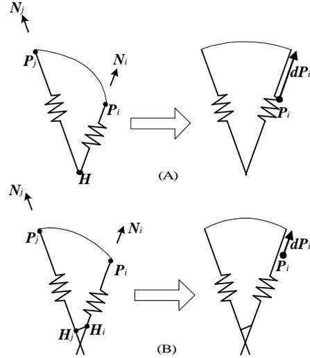
Figure 2: Definition of the spring model. (A) Displacement  $dP_i$  for a planar curve. (B) Displacement  $dP_i$  for a non-planar curve or a surface.
