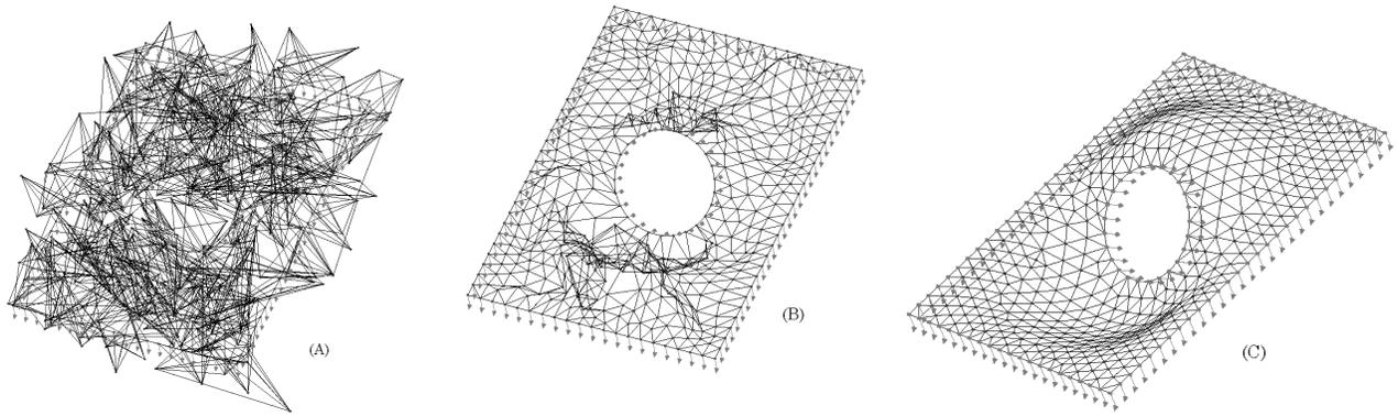
Figure 8: Stability of the algorithm. (A) Initial mesh with random noise on the nodes. (B) Shape (A) after five iterations of pre-smoothing on the finest level. (C) Shape (A) after full convergence.
