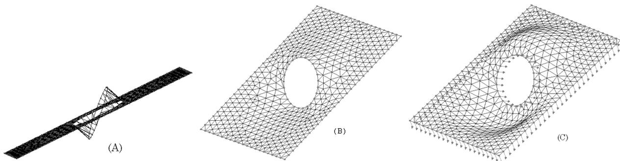
Figure 7: (A) Initial mesh. (B) Deformed result from (A) under the positional constraints on inner- and outer-boundary nodes. (C) Deformed result from (A) under the positional and normal constraints on inner- and outer-boundary nodes. Arrows on boundary nodes show the directions of normal constraints.
