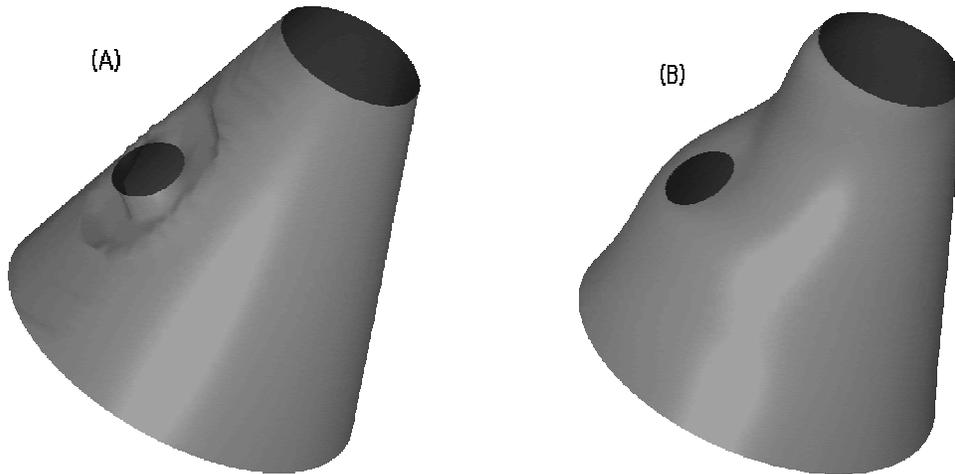
Figure 9: Shaded image of a deformed result. (A) Initial mesh. (B) Deformed result from (A) under the positional and normal constraints on nodes of upper-, lower-, and inner-boundaries.
