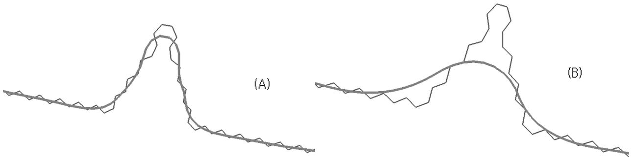
Figure 10: Least-square fitting of a polygonal segment to scattered points. A noisy thin line represents an initial segment. A smooth thick line represents a converged segment. Node positions of the initial segment are given as scattered points. (A) All weights  $k_j$  in Equation (11) are set to 0.01. (B) All weights  $k_j$  are set to 0.00001.
