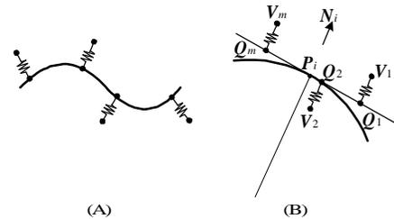
Figure 6: Least-square fitting of a planar curve to scattered points. (A) Geometric interpretation of general least-square fitting. (B) Geometric interpretation of our fitting approach.
