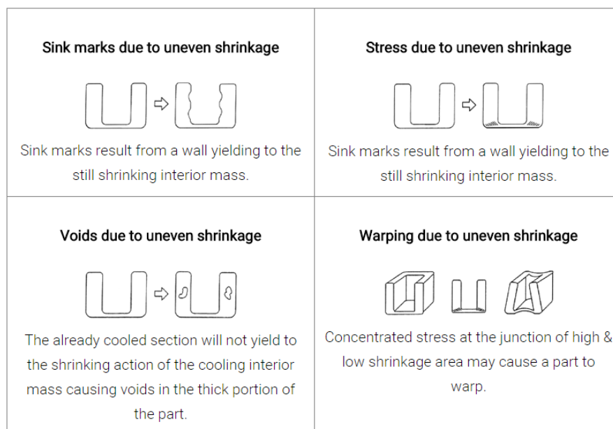
Figure 10.7: Uneven wall thickness leads to uneven shrinkage which can cause sinking, residual stress, voids or warping. Image from Plastics One.
