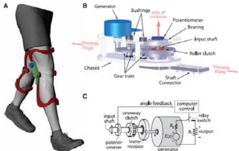
The diagram illustrates a prosthetic leg mechanism. Part A shows a 3D model of a prosthetic leg attached to a person's thigh. Part B is a detailed view of the mechanical assembly, including a generator, gear train, potentiometer, roller clutch, and shaft connector. Part C is a block diagram showing the control system, including an input shaft, potentiometer, transmission, generator, computer control, and relay switch.
