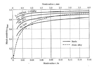
torsion. In using these charts it is well to know that the actual test results from which the curves were derived exhibit a large amount of scatter. Because of this scatter it is always safe to use  $K_f = K_t$  if there is any doubt about the true value of q. Also, note that q is not far from unity for large notch radii.
