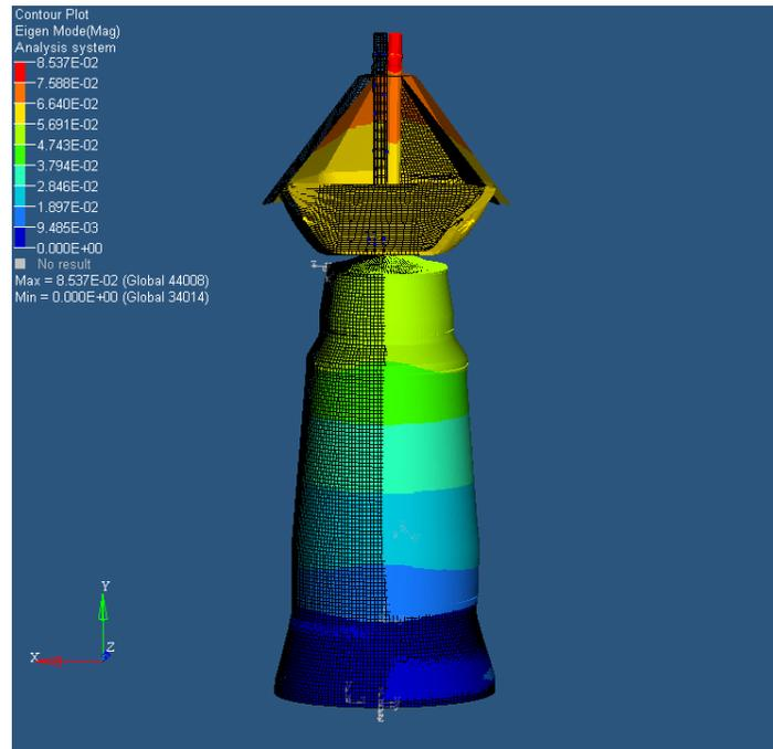
Figure 7: Displacement plot of Optistruct result, 1<sup>st</sup> lateral mode of vibration
