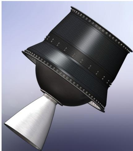
Figure 2: Braking interstage
