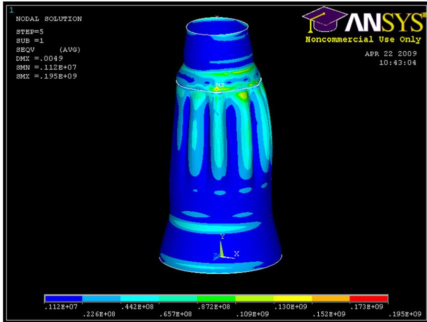
Figure 6: Stress plot of random vibration result
