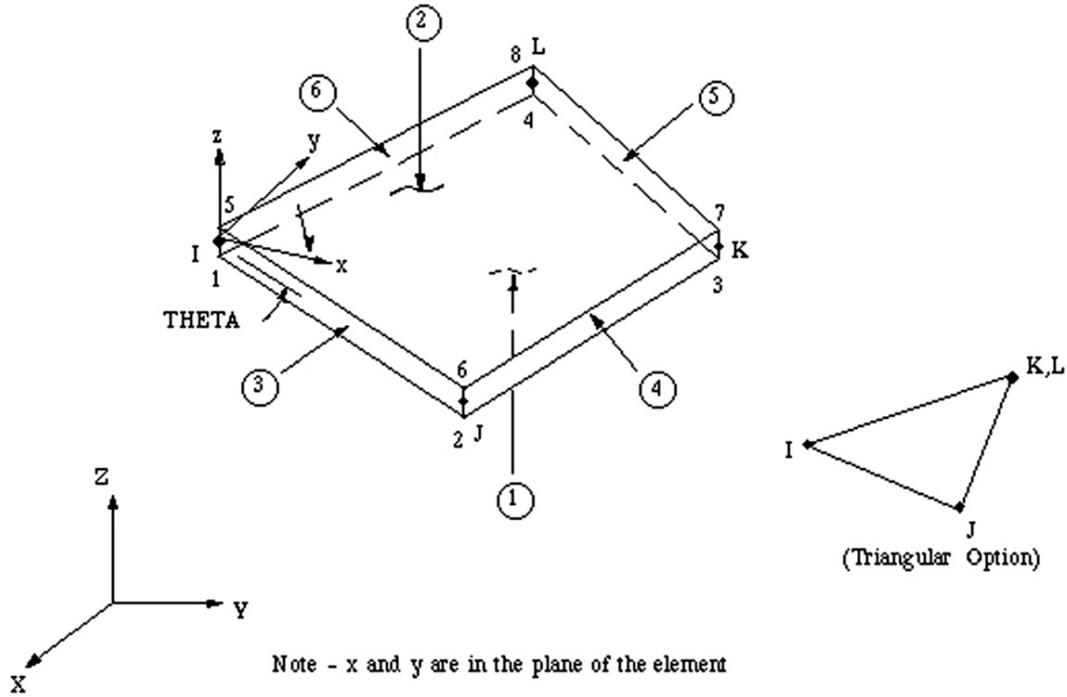
Fig. 1. Shell-63 element, elastic shell.
