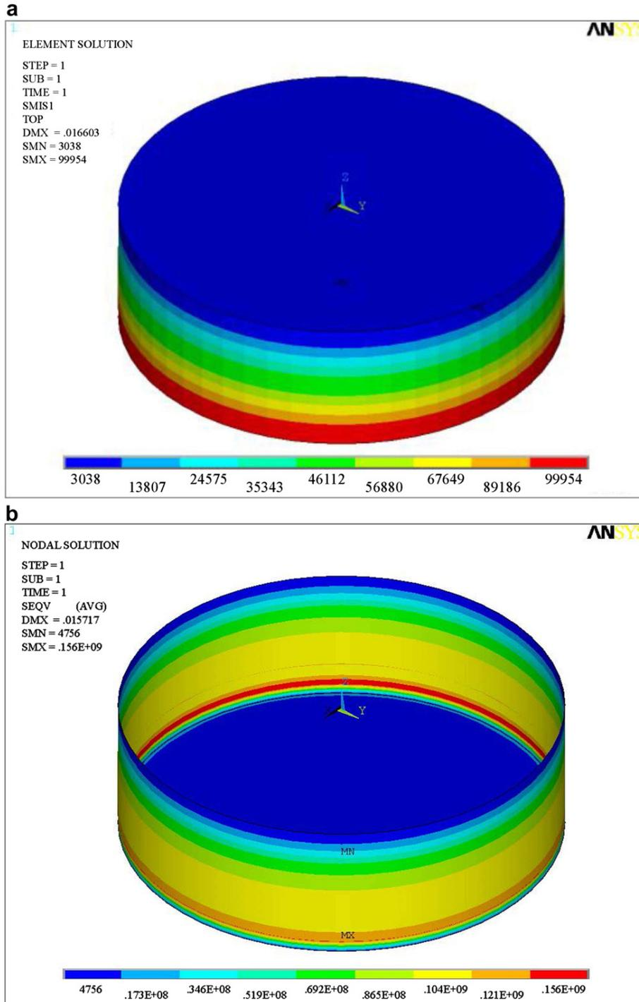
**Fig. 5.** A) hydrostatic pressure distribution at fluid element (mean value at the center of element), b) Von Mises stresses at the shell of tank due to static loading.
