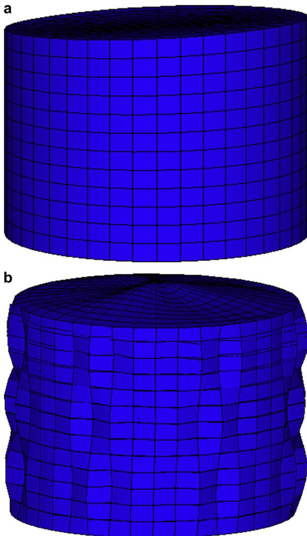
Fig. 3. Storage tank modal shape: a) convective mode, b) impulsive mode.
