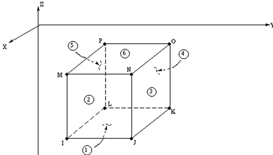
Fig. 2. Fluid-80, 3-D contained fluid element.
