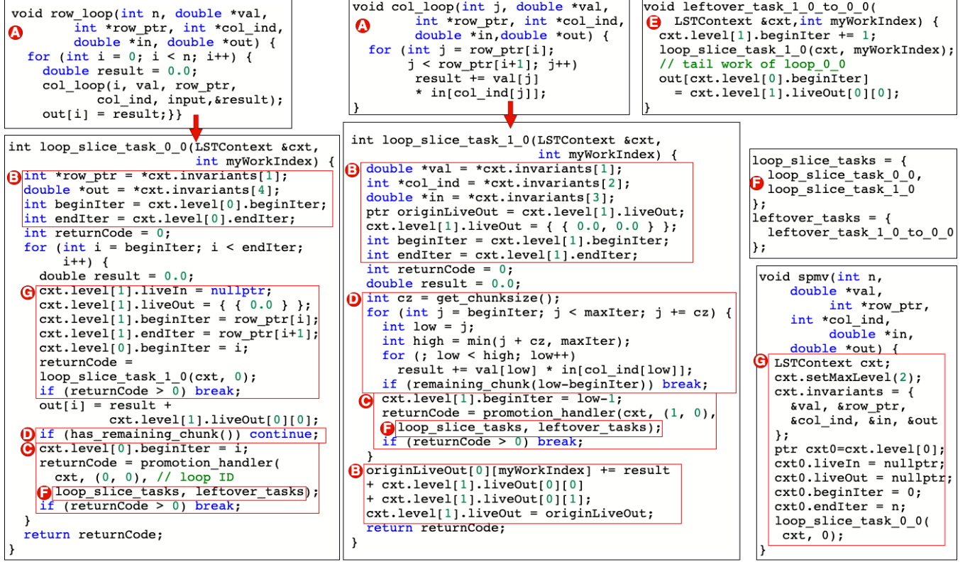
Figure 3. Sequence of transformations of spmv that are performed by the HBC’s middle-end. We used C++ code for readability and illustrative purposes. HBC performs these transformations in LLVM IR. The white letter in a red circle attached to the code surrounded by a rectangular red box indicates where in the pipeline of Fig. 2 that code is added.
