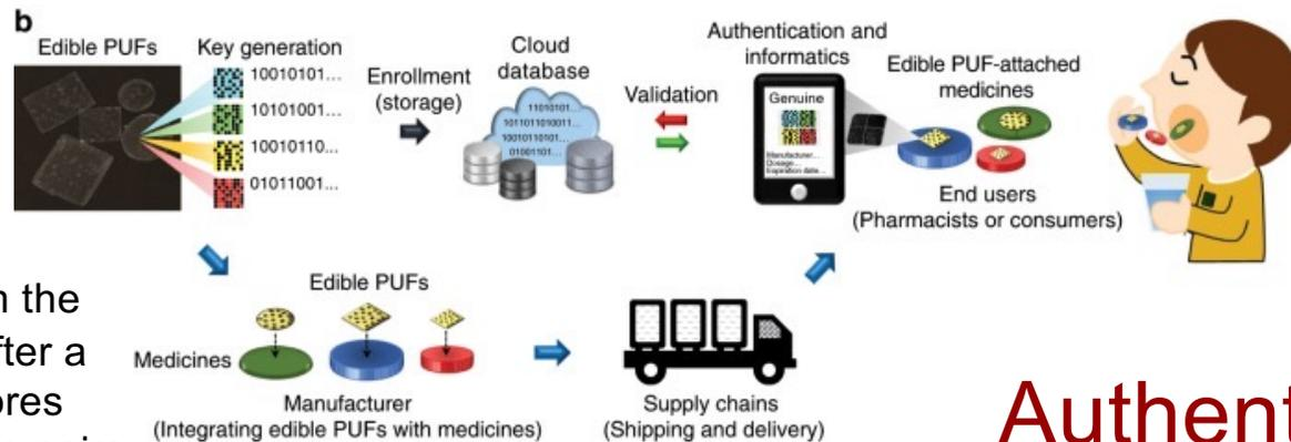
Delete the key from the secure database after a scan. Database stores challenge, response pairs.
