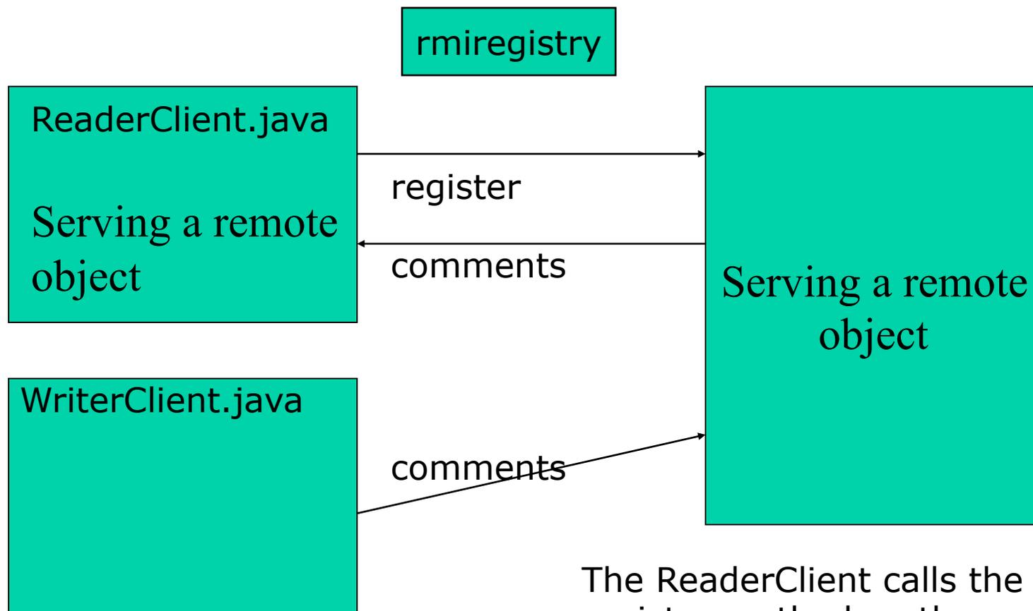
The ReaderClient calls the register method on the server side remote object. It passes a remote object reference.
