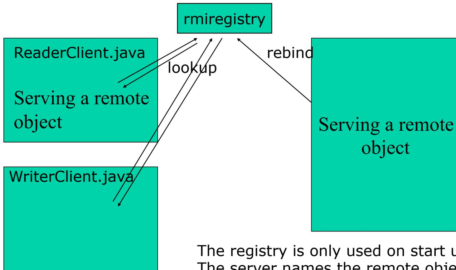
The registry is only used on start up. The server names the remote object and each type of client does a single lookup.
