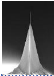
High Density Carbon tip (Nano Tools)
