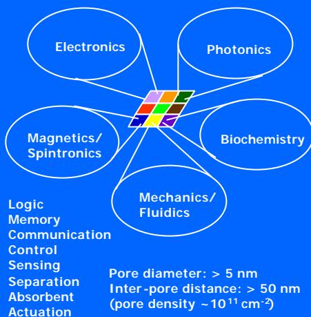
Nanopore arrays formed on silica with a directed self-organization method
