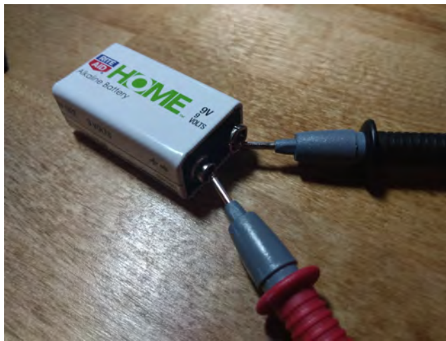
Figure 5: Measuring battery voltage
