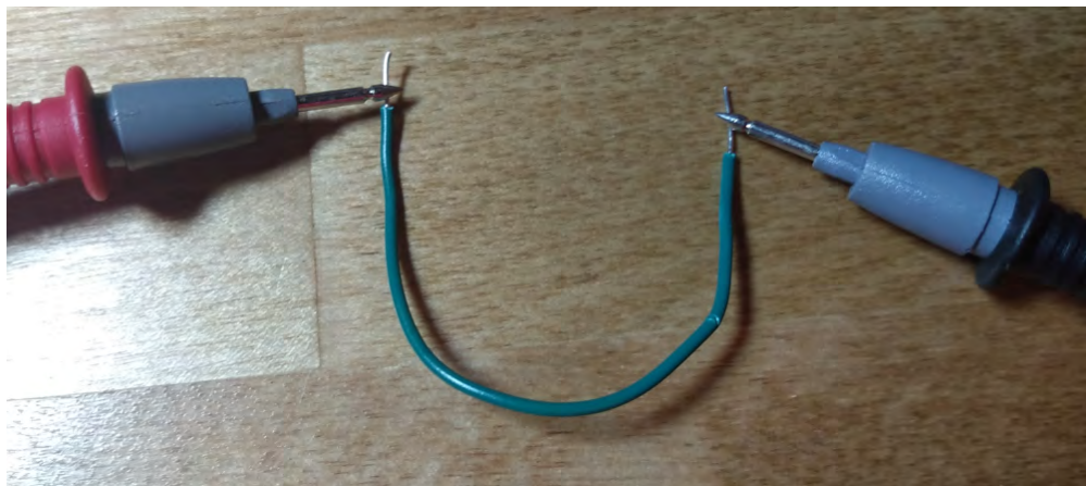
Figure 3: Testing the continuity of the wire with a digital multimeter.
