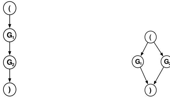
Figure 3: DAGs for sequential (left) and parallel (right) composition of two evaluated expressions e_1 and e_2 where G_1 and G_2 correspond to the DAGs of e_1 and e_2 respectively.
