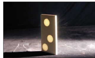
figure 4. gypsum board with resin pucks
