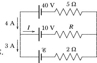
3. As I mentioned in lecture, we can apply Kirchhoff's rules to more complicated circuits. For example, here is a circuit with two batteries and three resistors,
