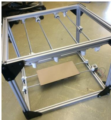
Figure 1: Frame assembly with rail and linear bearings attached.
