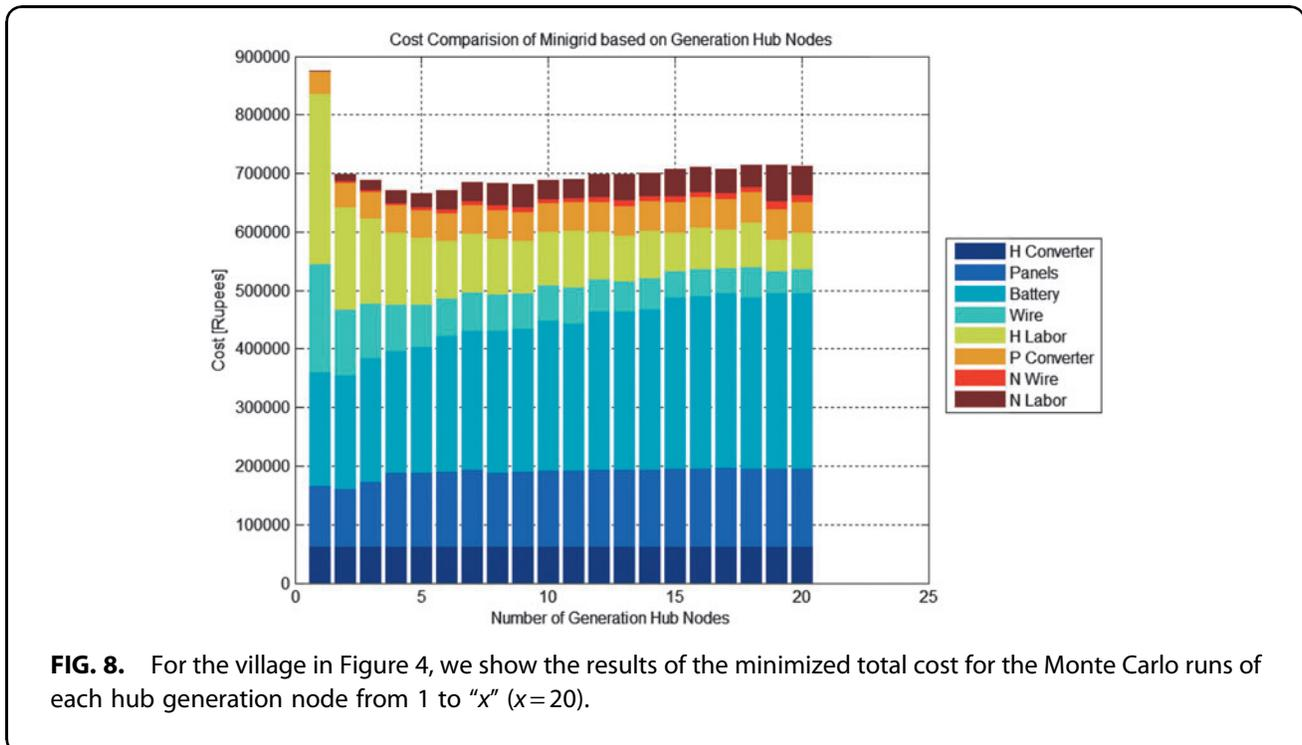
cost range. These variables are sampled in parametric space via a Monte Carlo method and the wiring costs are estimated via straight-line distances between points mated with a minimum spanning tree to connect a higher voltage-level architecture between nodes. Figure 8 shows the minimization curve of the total village cost for a given number of hub generation nodes.
