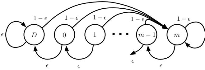
Fig. 3. The one dimensional random walk defined for the Buffer Refill scheme with finite buffer size and memoryless transition probabilities as depicted in the figure.
