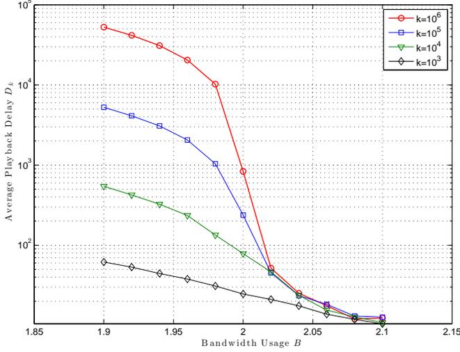
Fig. 2. The bandwidth-delay trade-off for different values of stream length  $k$ , and  $\epsilon = 0.5$ . This figure shows the transition in the behaviour of playback delay at  $B = \frac{1}{(1-\epsilon)} = 2$ .
