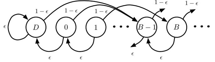
Fig. 1. The one dimensional random walk defined on the set of states  $S$  with infinite buffer size, fixed bandwidth usage  $B$ , and memoryless transition probabilities as depicted in the figure.
