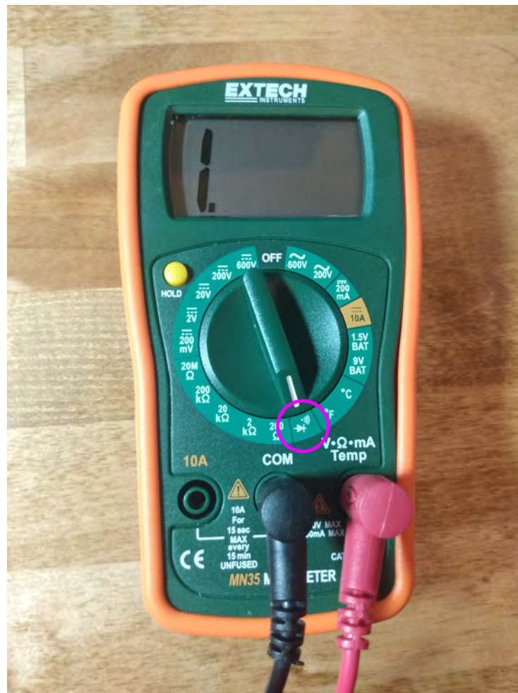
Figure 1: Selecting the continuity tester on the digital multimeter
