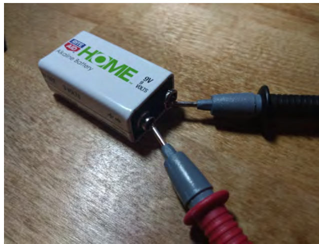
Figure 5: Measuring battery voltage
