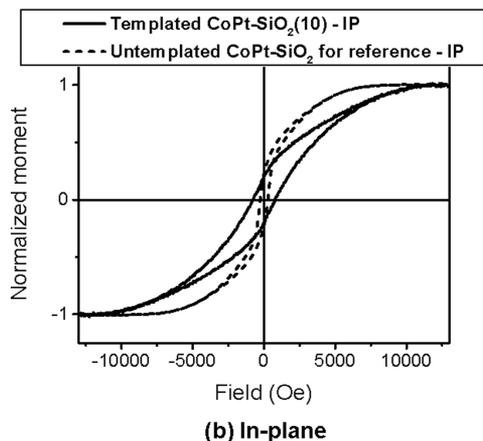
**Figure 3.** (a) Out-of-plane and (b) in-plane magnetic hysteresis loops for templated (solid line) and untemplated (dashed line) CoPt-SiO<sub>2</sub> magnetic media.
