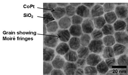
**Figure 4.** Plane-view transmission electron micrograph of templated CoPt-SiO<sub>2</sub> magnetic media.
