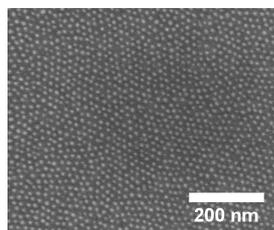
**Figure 2.** Plane-view scanning electron micrograph of am-C pillars after reactive ion etching.
