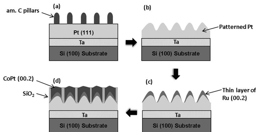
**Figure 1.** Illustration of process flow for fabrication of templated magnetic media showing film stack (a) after fabrication of am-C pillars, (b) after pattern transfer into template layer, (c) after sputtering underlayer, and (d) after sputtering magnetic layer with segregant.
