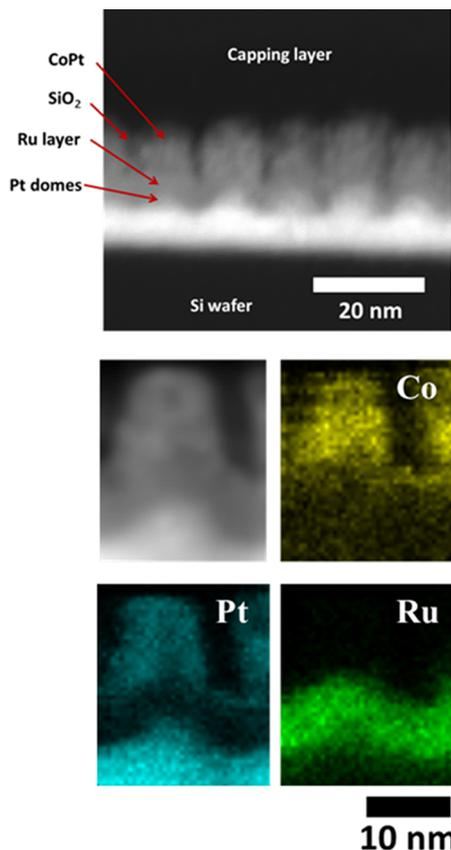
**Figure 5.** (a) High-angle annular dark field scanning transmission electron micrograph of templated CoPt-SiO<sub>2</sub> magnetic media. (b) EDS integrated intensity maps of Co, Pt, and Ru for one grain.
