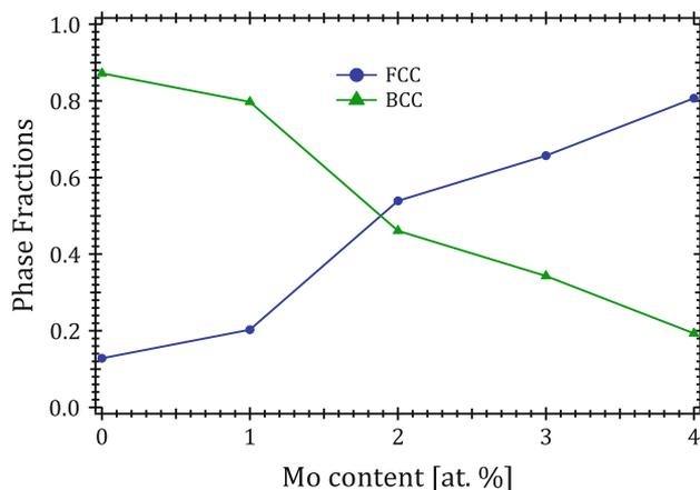
Fig. 2. Fractions of bcc and fcc phases in as-milled (Fe<sub>70</sub>Ni<sub>30</sub>)<sub>100-x</sub>Mo<sub>x</sub> ( $x = 0$  to 4) alloys, determined by x-ray diffractometry.
