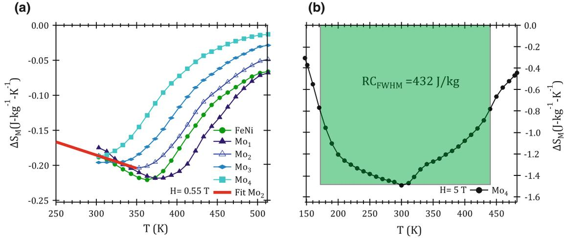
Fig. 3. Temperature dependence of the magnetic entropy change,  $\Delta S_M$ , of (a) solution-annealed  $(\text{Fe}_{70}\text{Ni}_{30})_{100-x}\text{Mo}_x$  ( $x = 0$  to 4) at 0.55 T (data for FeNi adapted from Ref. 6) and (b) solution-annealed  $(\text{Fe}_{70}\text{Ni}_{30})_{96}\text{Mo}_4$  at 5 T.
