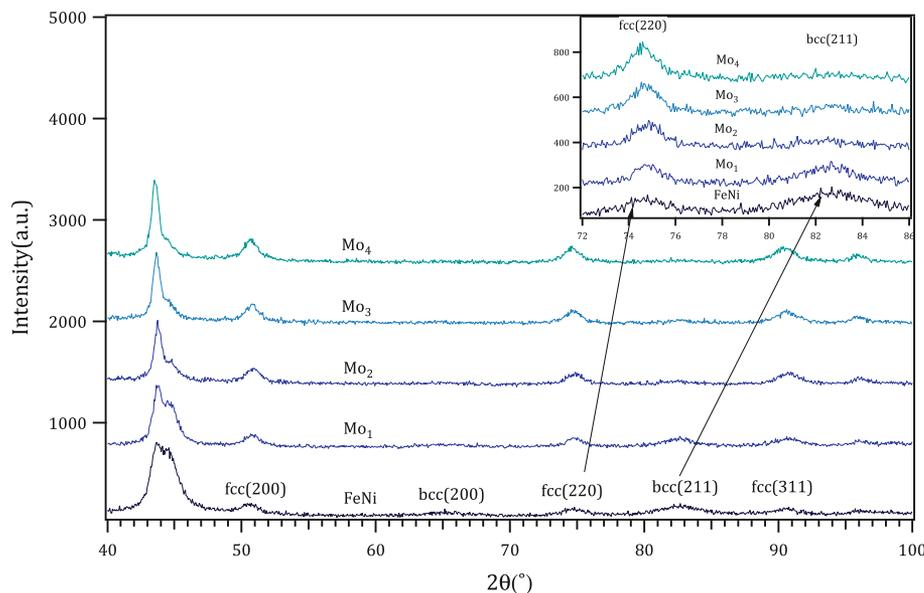
Fig. 1. x-Ray diffraction patterns of as-milled  $(\text{Fe}_{70}\text{Ni}_{30})_{100-x}\text{Mo}_x$  ( $x = 0$  to 4) alloys, labeled FeNi,  $\text{Mo}_1$ ,  $\text{Mo}_2$ ,  $\text{Mo}_3$ , and  $\text{Mo}_4$ , respectively. Inset: fcc(220) and bcc(211) peaks of as-milled  $(\text{Fe}_{70}\text{Ni}_{30})_{100-x}\text{Mo}_x$  ( $x = 0$  to 4) alloys.
