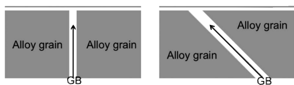
Figure 14. Schematic of the inclined GB to free surface.
