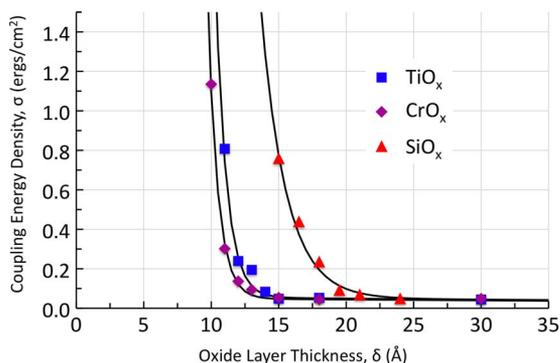
FIG. 4. (Color online) Coupling energy density as a function of oxide thickness for  $\text{SiO}_x$ ,  $\text{TiO}_x$ , and  $\text{CrO}_x$ .
