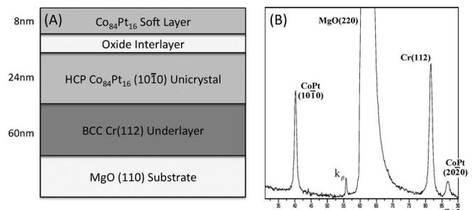
FIG. 1. (a) Structure of experimental model system. (b)  $\theta/2\theta$  XRD pattern of a Co<sub>84</sub>Pt<sub>16</sub> uniaxial.
