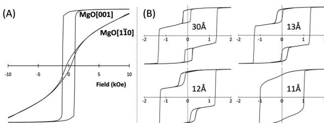
FIG. 3. (a) Uncrystal in-plane hysteresis loops measured along orthogonal MgO directions. (b) Example hysteresis loops showing exchange coupling with varying TiO<sub>x</sub> interlayer thickness.
