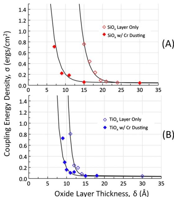
FIG. 5. (Color online) Comparison of coupling energy density with and without Cr dusting for (a)  $\text{SiO}_x$  and (b)  $\text{TiO}_x$ .
