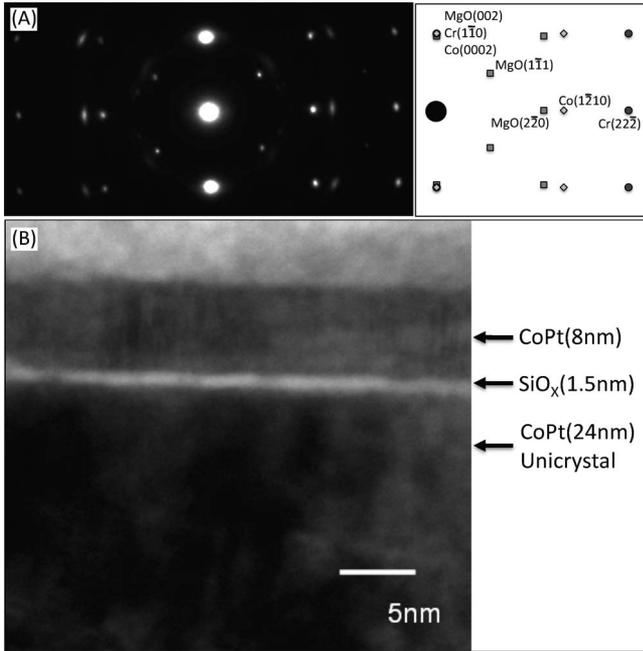
FIG. 2. (a) Plan view uncrystal electron diffraction pattern and predicted pattern w/indexing (right half shown only). (b) Cross-section TEM image showing CoPt layers with 1.5 nm SiO<sub>x</sub> interlayer.
