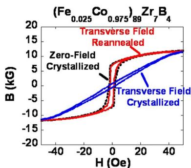
FIG. 4. (Color online) Dynamic  $B$ - $H$  loops for a  $(\text{Co}_{0.975}\text{Fe}_{0.025})_{89}\text{Zr}_7\text{B}_4$  alloy after zero-field crystallization (dashed, black) at  $T_{\text{anneal}}=540^\circ\text{C}$  followed by a transverse field reannealing treatment (solid, red) under the same annealing conditions and compared to a transverse field crystallized ribbon at  $T_{\text{anneal}}=540^\circ\text{C}$  (solid, blue).
