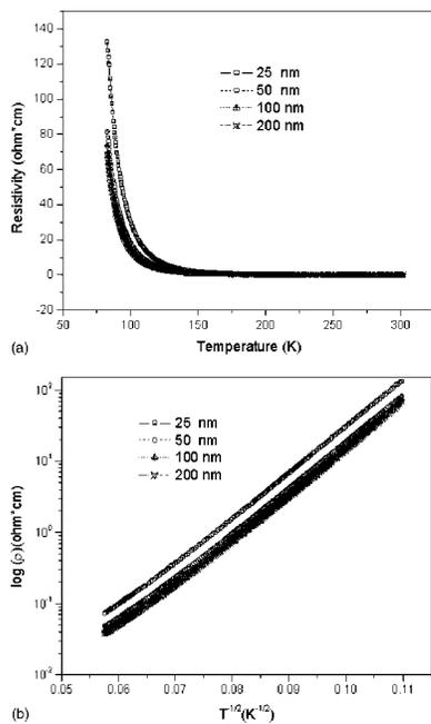
FIG. 3. Resistivity vs (a) temperature and (b)  $T^{-1/2}$  for the films grown at room temperature as a function of thickness.
