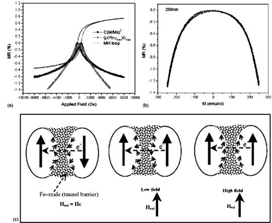
FIG. 4. (a) Magnetoresistance, hysteresis, and  $-(M/M_s)^2$  curves vs applied field, (b) magnetoresistance vs magnetization for a 200-nm Fe<sub>3</sub>O<sub>4</sub> film, and (c) schematic model for the MR behaviors. The measurement was conducted at 300 K.
