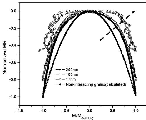
FIG. 6. Magnetoresistance curve measured at room temperature for  $\text{Fe}_3\text{O}_4$  films at different thicknesses. Magnetization is normalized by magnetization at 5500 Oe.
