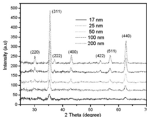
FIG. 1. In-plane XRD patterns as a function of film thickness at an oxygen flow rate of 6.8 SCCM and Ar flow rate of 27 SCCM.
