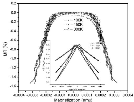
FIG. 5. Magnetoresistance vs magnetization of a 17-nm Fe<sub>3</sub>O<sub>4</sub> film at various temperatures. The inset shows the magnetoresistance as a function of field.
