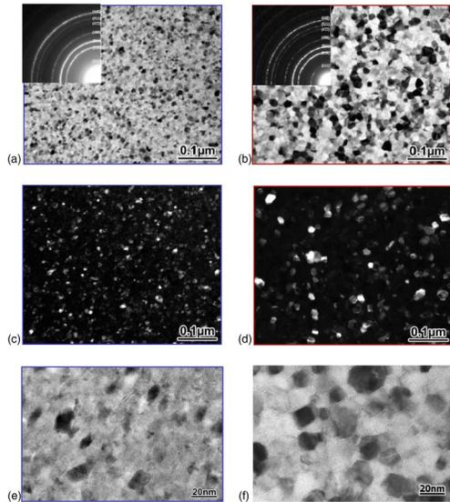
FIG. 2. (a) Bright field, (c) dark field, and (e) magnified images of 17 nm, and (b) bright field, (d) dark field, and (f) magnified images of a 100-nm Fe<sub>3</sub>O<sub>4</sub> film. SAD is shown in the upper corner of the bright field image.
