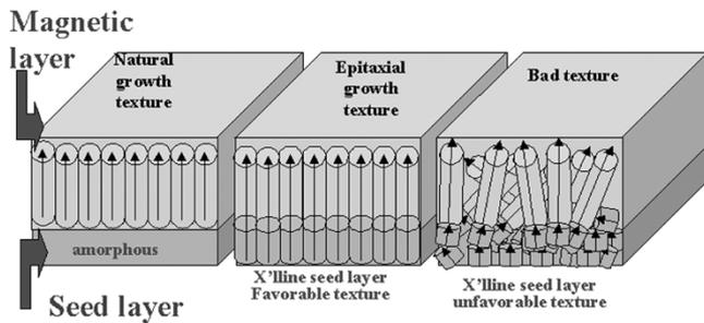
Fig. 2. Schematic representations of the growth of Co grains on different intermediate layer structures.
