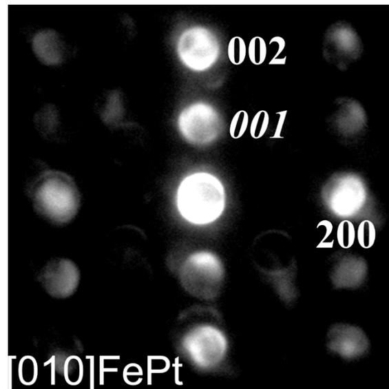
Fig. 7. A nano beam electron diffraction pattern of L1<sub>0</sub> FePt thin film taken in cross section. The film has perpendicular texture.
