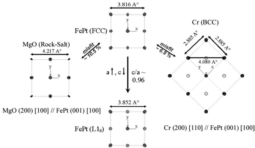
Fig. 8. The epitaxial matching of the FePt lattice with the MgO and the Cr lattices can be used to promote the (001) textured growth of FePt thin films.
