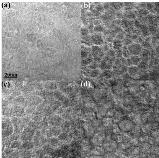
Fig. 5. EELS spectra of Co alloy media: (a) is zero energy loss spectrum, (b), (c), and (d) are Cr, Mn, and Co mapping of (a), respectively.
