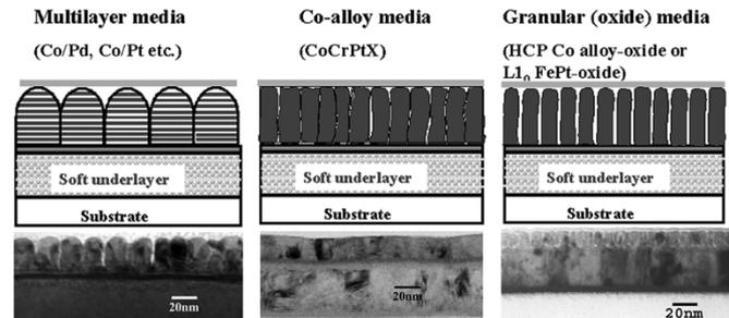
Fig. 1. Schematic structures and cross section microstructures of three types of perpendicular media.
