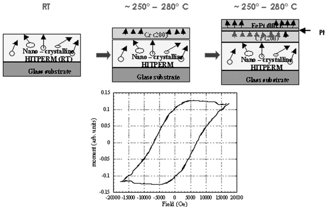
Fig. 9. Schematic representation of the growth of (002) textured FePt on Cr (200) seed layers and with a soft underlayer. Cr develops the required (200) texture only over a narrow range of temperatures. The hysteresis loop was obtained using the anomalous Hall effect. The film structure was Fe-Pt (30 nm)/Pt (3 nm)/Cr (80 nm)/HITPERM (100 nm)/glass substrate.
