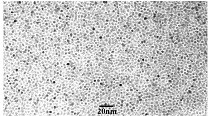
Fig. 3. Granular media displaying 3.5 nm grains.
