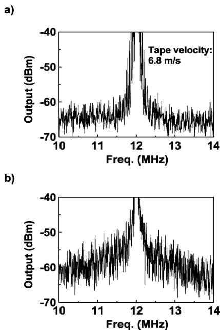
Fig. 4. Spectrum of 90 kfcI density signal. The sidebands of the fundamental component of the sputtered tape media deposited on (a) a smooth base film (ARAMID) and (b) a conventional base film (PEN). The RBW of the measurement was 10 kHz.
