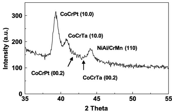
Fig. 3. The X-ray diffraction spectrum shows a weak Co (00.2) peak along with a strong Co (10.0), indicating the prominence of (10.0) texture.
