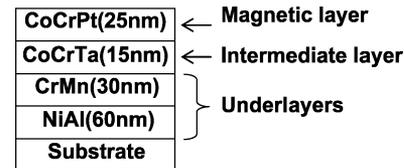
Fig. 1. Typical sample structure: substrate/NiAl (60 nm)/CrMn (30 nm)/CoCrTa (15 nm)/CoCrPt (25 nm).
