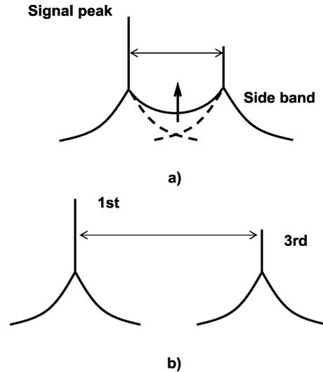
Fig. 8. Illustration of spectral plot of amplitude modulation sideband noise. For lower recording density, less separation between the fundamental harmonics occurs, yielding folded sidebands between the two harmonics. (a) Long wavelength. (b) Short wavelength.
