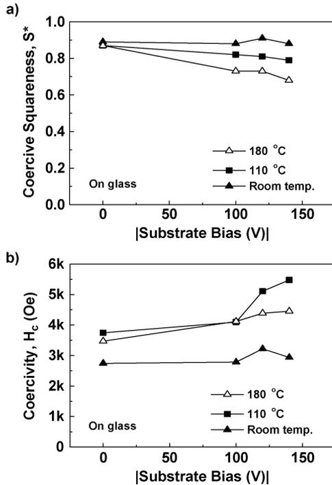
Fig. 10. The variation of magnetic properties of the CoCrPt media on glass versus substrate bias and temperature: a)  $S^*$  and b)  $H_c$ .
