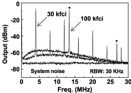
Fig. 7. Spectrum for recording square wave. The broad-band noise level increases at higher recording density.
