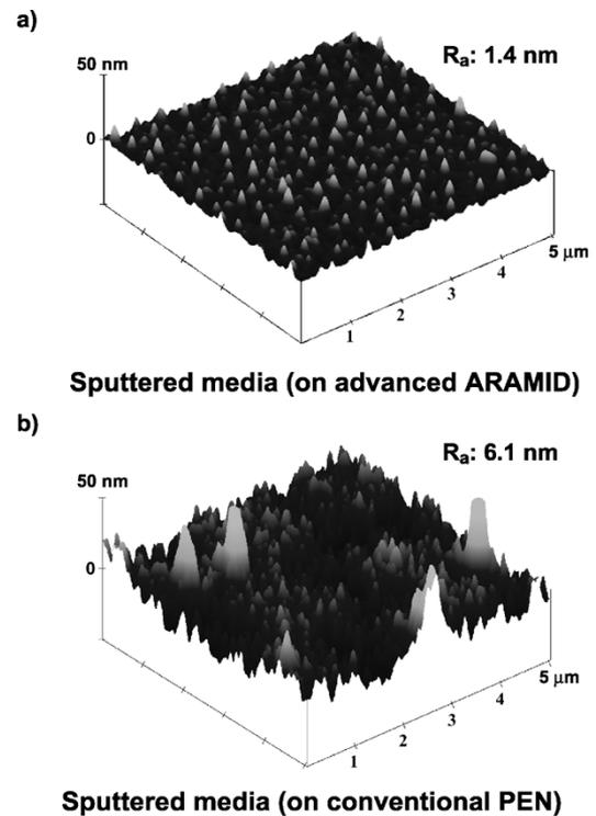
Fig. 5. Measured roughness properties of sputtered media on (a) advanced ARAMID with  $R_a$  of 1.4 nm and (b) conventional PEN with  $R_a$  of 6.1 nm.
