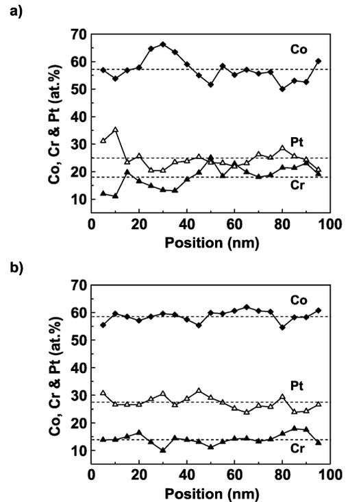
Fig. 11. Variation of Co, Cr, and Pt concentration measured in a plan-view TEM image of the CoCrPt layer: (a)  $\text{Co}_{57}\text{Cr}_{16}\text{Pt}_{27}$  films bias-sputtered and (b)  $\text{Co}_{59}\text{Cr}_{15}\text{Pt}_{26}$  films sputtered without bias.
