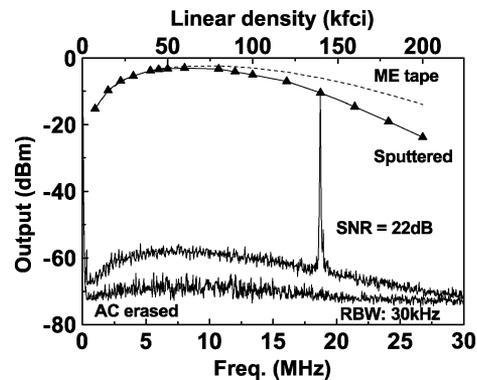
Fig. 9. Spectra of signal and noise for the sputtered tape media with the AMR head. The SNR showed about 22 dB at channel density ( $D_{50}$ ) of 140 kfcf. An experimental ME medium is also shown for comparison.
