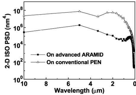
Fig. 6. Measured power spectral density and curve fitting for media (on advanced ARAMID) and media (on conventional PEN).
