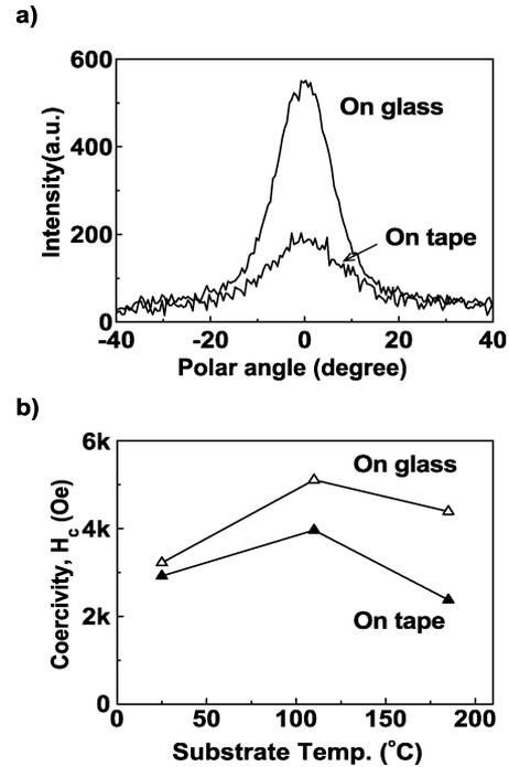
Fig. 2. Structural and magnetic properties of CoCrPt films on glass and tape (KAPTON) substrates: (a) rocking curves for (10.0) oriented media and (b) in-plane coercivity ( $H_c$ ) as a function of substrate temperature.
