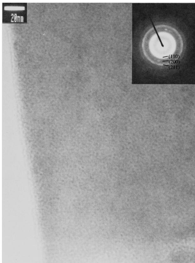
FIG. 2. Bright-field image and SAED pattern of 100 nm HITPERM film prepared at RT and under  $4.5 \text{ W/cm}^2$  sputter power density.
