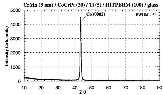
FIG. 5. XRD scan from a CrMn/CoCrPt/Ti/HITPERM film structure where the HITPERM was prepared at 4.5 W/cm<sup>2</sup> sputter power density. The CoCrPt layer shows a strong hcp (0002) orientation with a full width at half maximum distribution of  $\sim 5^\circ$  (determined from rocking curve measurements).
