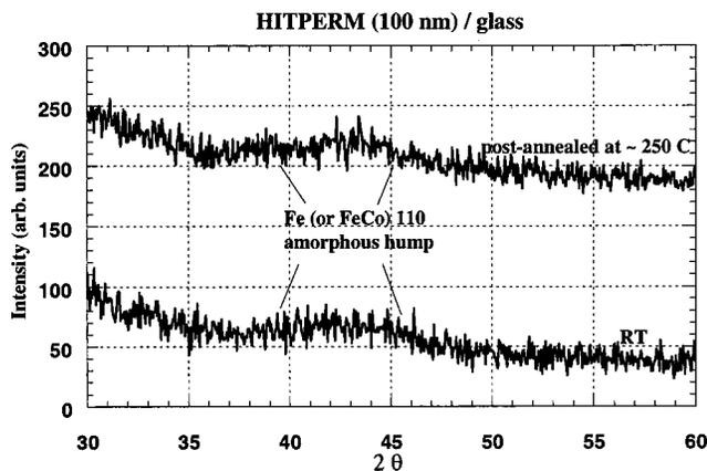
FIG. 1. XRD scans from HITPERM films sputtered onto glass substrates at  $4.5 \text{ W/cm}^2$  power density. While both films were prepared at RT, the top one was then annealed at  $\sim 250^\circ\text{C}$  for 30 min.
