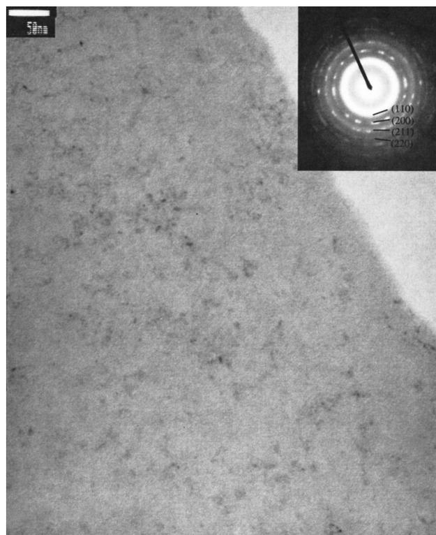
FIG. 3. Bright-field image and SAED pattern of 100 nm HITPERM film prepared at RT and under  $4.5 \text{ W/cm}^2$  sputter power density after annealing in-situ at  $\sim 250^\circ\text{C}$  for 30 min.
