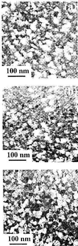
Fig. 5. Plan-view dark-field TEM images of CoCrPt films in the NiAl/CrMn/CoCrPt (a), NiAl/CrMn/CoCrTa/CoCrPt (b) and the NiAl/CrMn/CoCrMn/CoCrPt (c) tape media. The CoCrPt films in both NiAl/CrMn/CoCrPt and NiAl/CrMn/CoCrTa/CoCrPt tape media contain many grains with size less than 8 nm whereas the CoCrPt grains in the NiAl/CrMn/CoCrMn/CoCrPt tape medium are more uniform in size.
