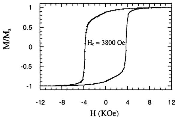
Fig. 3. In-plane magnetic hysteresis loop of the NiAl/CrMn/CoCrMn/CoCrPt tape medium (structure d). The coercivity of this medium is around 3800 Oe.
