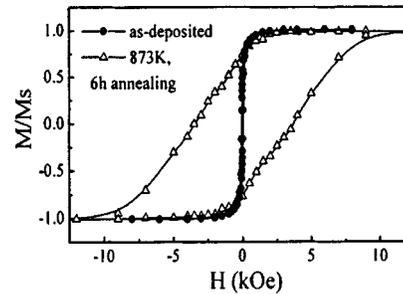
Fig. 4. In-plane hysteresis loops for  $a\text{-Al}_2\text{O}_3/\text{Fe}/\text{Pt}$  films on (100) NaCl substrate (unannealed and annealed at 873K for 6 h).
