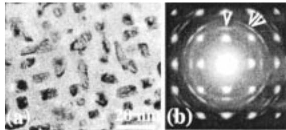
Fig. 1. TEM image and SAED pattern of a- $Al_2O_3$ /Fe/Pt film. The 002 and 112 reflections of  $\alpha$ -Fe are marked by single and double arrows respectively in (b).
