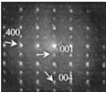
Fig. 3. NBD pattern of local region of a FePt particle. The  $c$ -axis of the FePt region is in the film plane and the  $c/a$  ratio was approximately 0.97.
