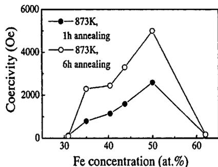
Fig. 6. Composition dependence of magnetic coercivity of 873K annealed a-Al<sub>2</sub>O<sub>3</sub>/Fe/Pt films.
