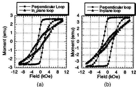
FIG. 2. In-plane and perpendicular  $MH$  loops for (a) sample A and (b) sample B.
