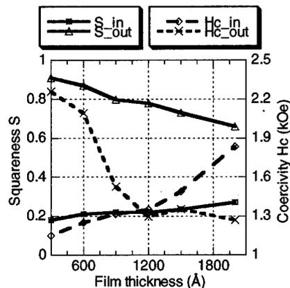
FIG. 1. Film thickness dependence of in-plane squareness  $S_{in}$ , perpendicular squareness  $S_{out}$ , in-plane coercivity  $H_{c,in}$ , and perpendicular coercivity  $H_{c,out}$  for single layer BaM thin films.
