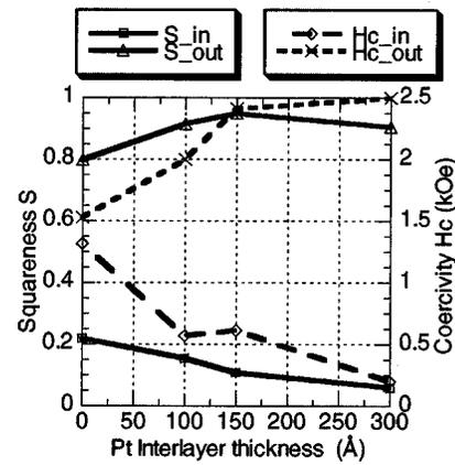
FIG. 3. Pt interlayer thickness dependence of  $S_{in}$ ,  $S_{out}$ ,  $H_{c_{in}}$ ,  $H_{c_{out}}$ . The structures of all BaM films are the same as sample B except for the variation in Pt thickness as noted.
