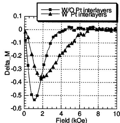
FIG. 4.  $\delta M$  curves for samples A and B measured by VSM.
