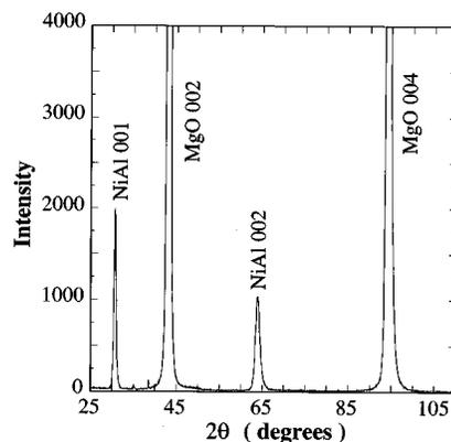
FIG. 1. The x-ray diffraction spectrum of the  $\text{Co}_{72}\text{Cr}_{10}\text{Pt}_{18}/\text{NiAl}/\text{MgO}/(001)\text{MgO}$  film.
