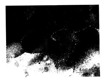
FIG. 1. Bright field TEM micrograph of garnet film annealed in a conventional furnace at  $670~^{\circ}\text{C}$  for 3 h in an air atmosphere.
