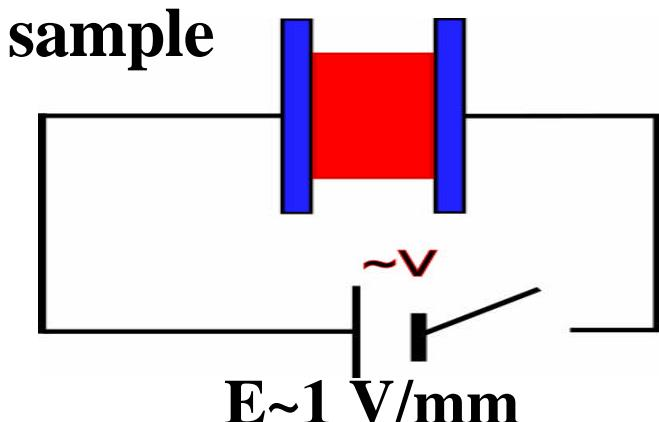
DS measures the relation between time-varying voltage and current through a sample
