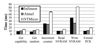
Figure 9. Mean time for various TPM operations. Error bars represent 95% confidence intervals.
