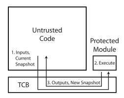
Figure 1. **Execution Model.** The Trusted Computing Base (TCB) isolates the protected module from untrusted code. Memoir securely maintains state continuity for the protected module, despite relying on the untrusted code for bulk persistent storage.
