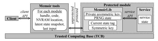
Figure 2. Architecture of Memoir. Rounded boxes indicate persistent storage.
