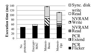
Figure 10. Breakdown of mean request execution time for the Noop module. Legend excludes parts so short as to be invisible. Error bars, some of which are too small to see, represent 95% confidence intervals.
