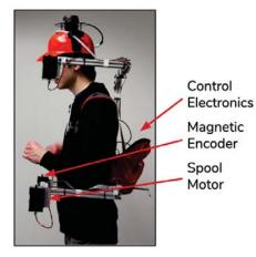
Figure 5: Electronics subsystems in context.
