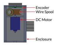
Figure 4: Schematic of one of In-Sight's three wire spools.
