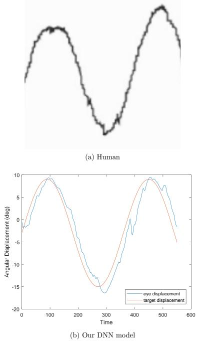
Figure 5.14: Plot of eye transition in smooth pursuit tracking a visual target, which moves with a sinusoidal curve in the horizontal direction. The plot shows the ocular angular displacement (blue line) and the visual target (red line) over time.
