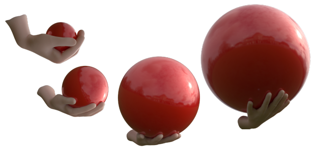
Fig. 9. Demonstration of a manipulator adapting its grip in response to variance in object scale.
