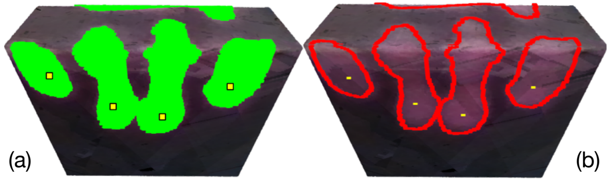
Figure 4.2: Illustration of the boundary model and its associated parameterization entities, including the (yellow) root in relation to (a) the original areas in green and (b) the boundary points in red.
