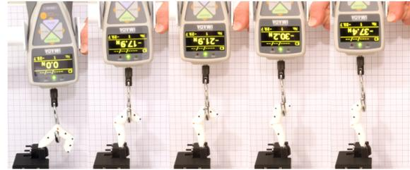
Figure 5: Individual finger strength test: In the flexed configuration, the finger withstands a maximum load of 37.4N.
