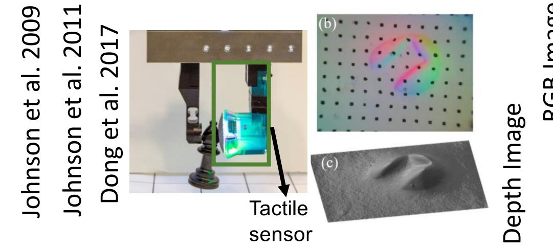
GelSight tactile sensor allows to capture dense tactile information which is essential for dexterous robot manipulation.
