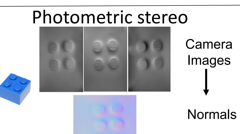
With photometric stereo, GelSight can encode surface normals as an RGB image.
