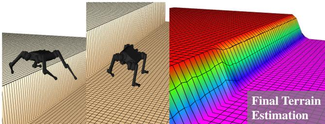
Fig. 6. Control behavior and terrain estimation results of the proposed proprioception-based gait planner when a robot walks sideways down an unforeseen cliff. Left: Proprioception recognizes the loss of contact, and the gait planner modifies the contact schedule and repositions the legs. Middle: With modified gait and controls, the robot lands in an appropriate posture. Right: The final terrain estimate successfully models stepped terrain.
