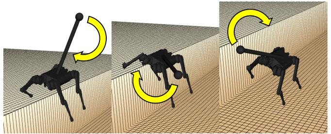
Fig. 7. Tailed robot control behavior with NMPC when falling off a cliff. The NMPC applies a conical motion that enables the tail to apply continuous torque to the body without hitting the joint limit.
