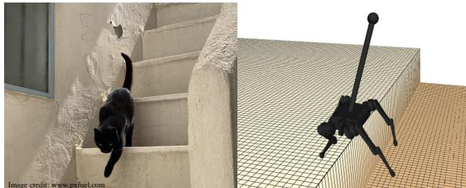
Fig. 1. A comparison of a cat and a quadruped robot with a tail walking over extreme elevation changes. Animals provide inspiration for the design, control, planning, and perception strategies of quadruped robots for traversing extreme terrains.
