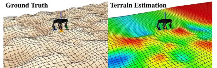
Fig. 4. Terrain estimation results obtained by simulating quadrupeds walking on rough terrain and using the proposed terrain estimation algorithm to model height variations without prior knowledge. Left: Ground truth. Right: Estimated terrain elevation.
