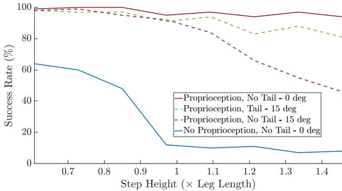
Fig. 5. Batch simulation success rate statistics under different initial conditions and environments.
