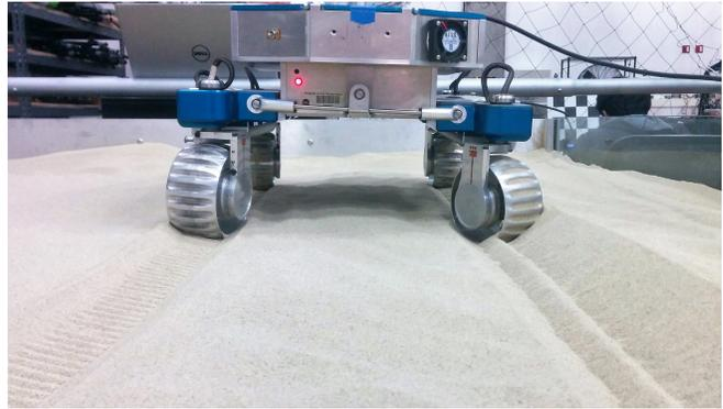
Fig. 1: K10 mini rover using its rear right wheel to trench. K10 mini is a microwave-sized rover from NASA Ames.
