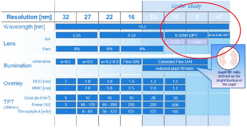
EUVL can be extended to sub-10 nm patterning using double patterning and/or high-NA EUV
