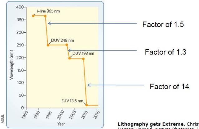
Figure 1 | Since the mid-1980s, the wavelength of light used in lithography systems has reduced by almost half from 365 nm to 193 nm. The switch to EUV lithography involves a further wavelength reduction factor of almost 15. DUV, deep ultraviolet. Lithography gets Extreme, Christian Wagener and Noreen Harned, Nature Photonics, Vol. 4, pp. 24-26, January 2010
