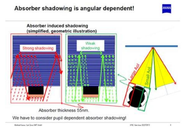
New mask structure including re-designed reflector and thin absorber is needed for high-NA system.
